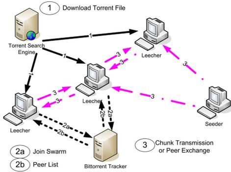
Figure 1: Typical operation of the BitTorrent protocol
