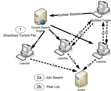
Figure 2: Using BitTorrent to generate a DDoS attack
